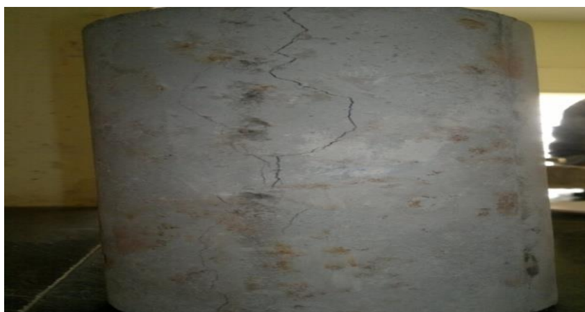
Fig -7: Crack along the length of cylinder.
