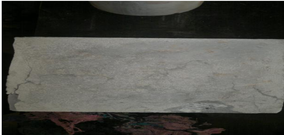
Fig -8: Crack propagating in cube.
