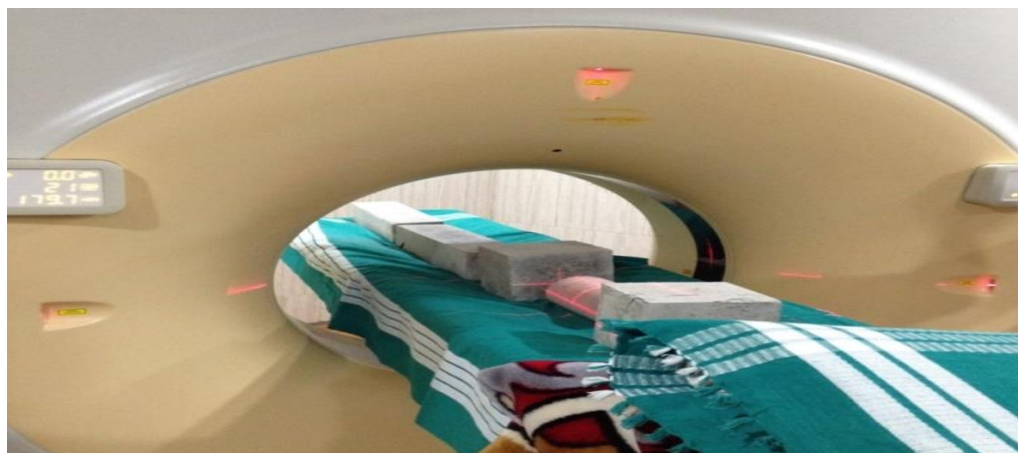
Fig -9: specimen kept for CT scanning
